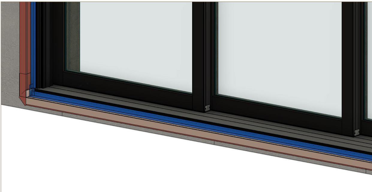
Exterior waterproofing detail
