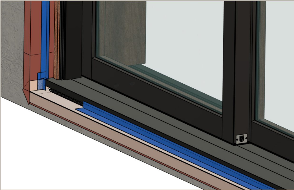
Exterior waterproofing detail
