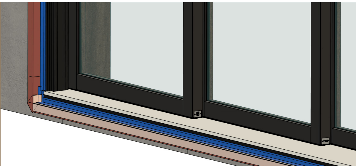
Exterior waterproofing detail
