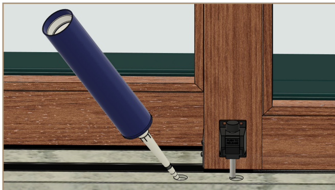
Application of the adhesive
